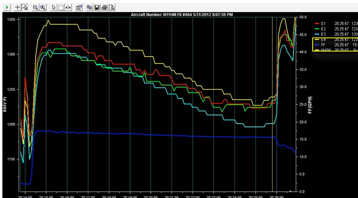
Figure 27:  $V_Y$  climb flight test data, M20J EGT and fuel flow, May 31, 2012. Full rich EGT as per Mooney M20J POH (1984). Yellow vertical line indicates fuel flow at  $V_Y$  top of climb, yellow box encloses fuel flow value (15.6 gallons per hour).
