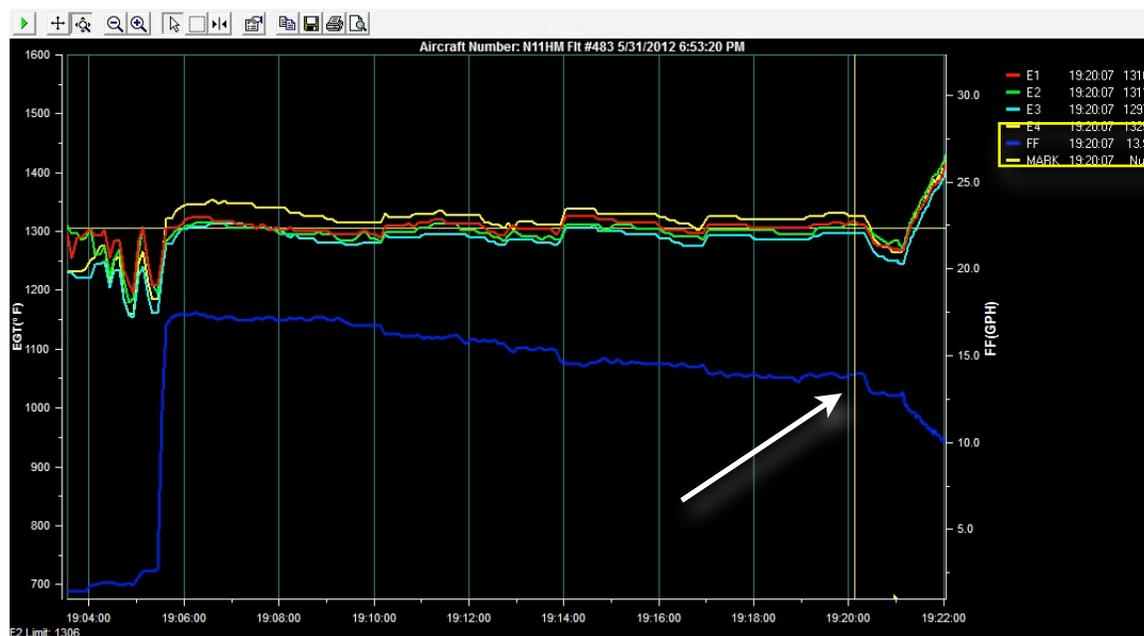
Figure 26:  $V_Z$  climb flight test data, M20J EGT and fuel flow, May 31, 2012. Target EGT method of mixture control. White arrow indicates fuel flow at  $V_Z$  top of climb, yellow box encloses fuel flow value (13.9 gallons per hour).
