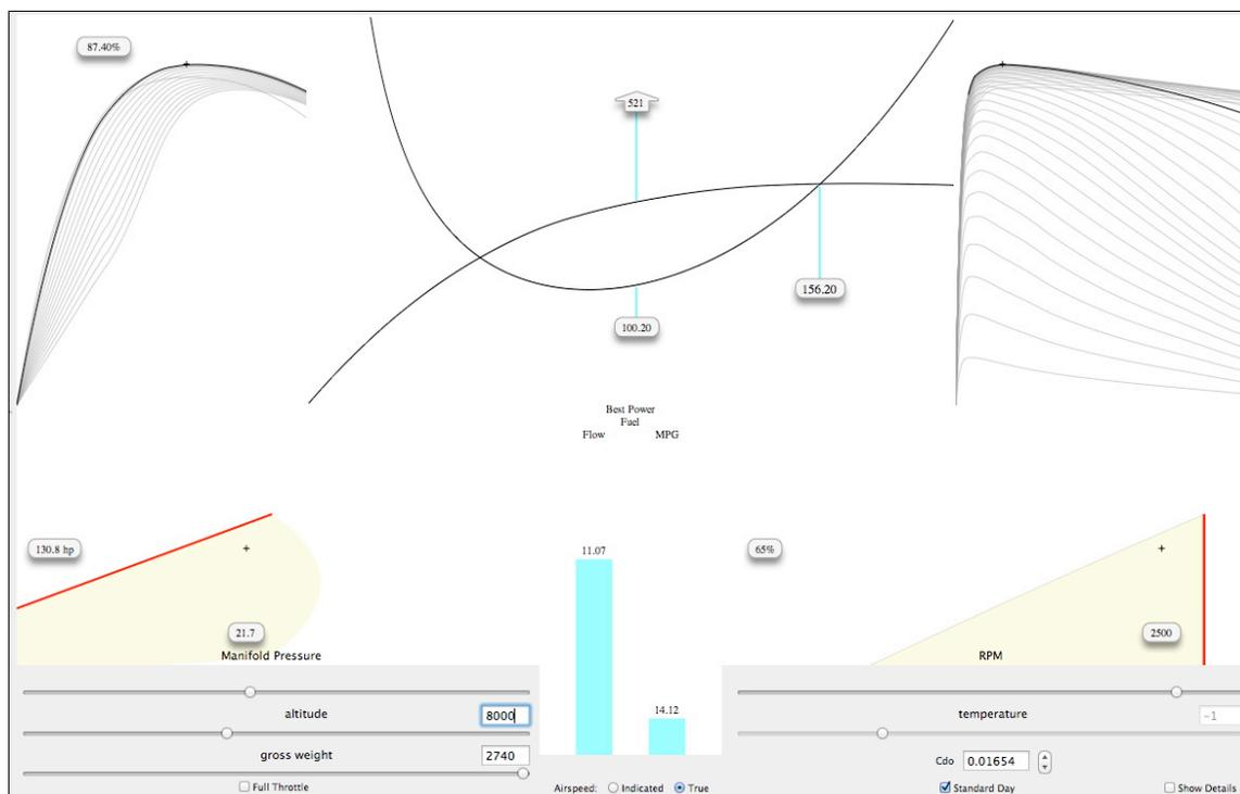
*Figure 16:* Benchmark airplane speed chart. Condition shown is a 65% power, best power mixture, cruise at 8000' pressure altitude, standard day for the Mooney M20J. Modeled true airspeed 156.2 knots (POH is 157 knots) and fuel flow is 11.08 gallons per hour (POH is 11.1 gallons per hour). These data were utilized for the values in Table 3, above.
