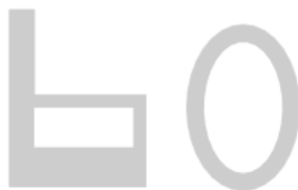
I_{xy} \neq 0 I_{xy} = 0 Product of Inertia
