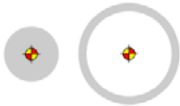
Polar Moment of Inertia These objects have equal section area but the hollow circle has a much larger polar moment of inertia.
